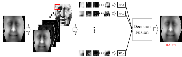
Figure 5. From head pose invariant face representation to the expression label (left to right): initial 2D face representation, channel computation, dense sampling with overlapping patches, random forest classification, decision fusion and labeled sample.
